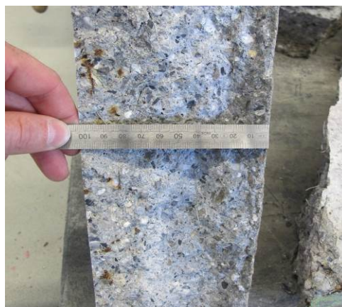
Figure 8 Photo of steel fiber reinforced square panel (A1) after 1 year of exposure to Salt (NaCl)-solution (3%) after square panel testing.
