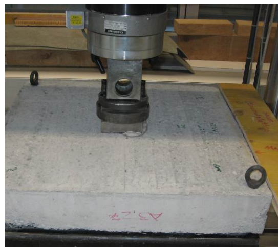
Figure 1 Crack production in interrupted EFNARC square panel test. Test was stopped at a deformation of 3 mm.
