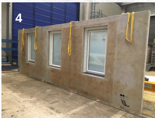
4 Strip the formwork and storage
