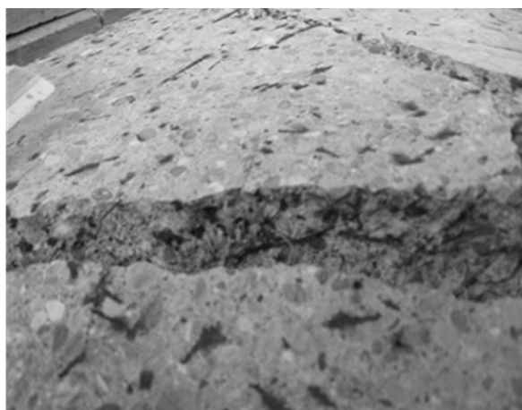
3% NaCl solution: steel fibres => very strong fibre corrosion (also inside the cracks)
