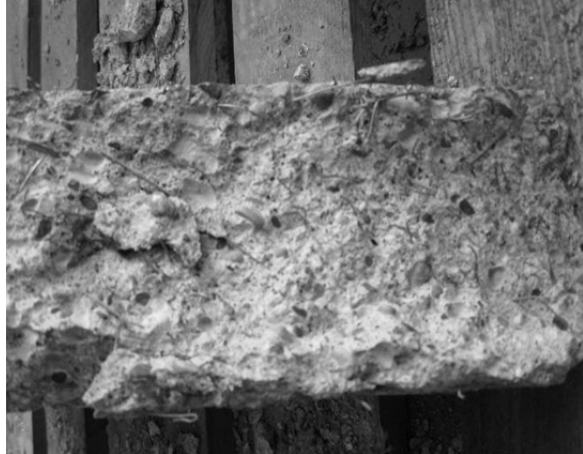
Free weathering: steel fibres => some fibre corrosion (mostly close to the surface)
